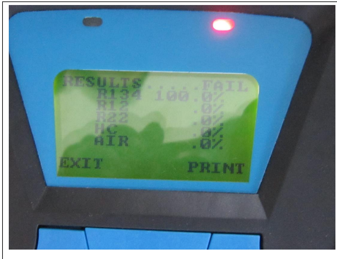
Fig.3: The analysis results on the screen of the ODS identifier from R134a-The results confirm that the cylinder has 100% R134a (R12-0%, R22-0%, HC-0% and Air-0%)
