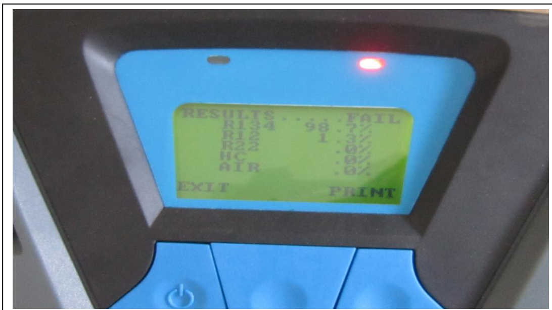
Fig. 4: The analysis results on the screen of the ODS identifier from R410A-The results confirm that the cylinder has 98.7% R134a and R12- 1.3% (R22-0%, HC-0% and Air-0%)
