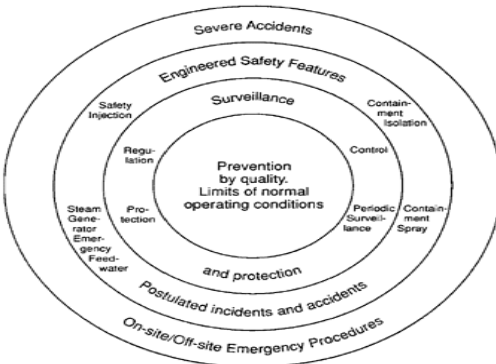
Figure 2-3: The protection levels in the design and operation of the nuclear power plant following the defence in depth principle
