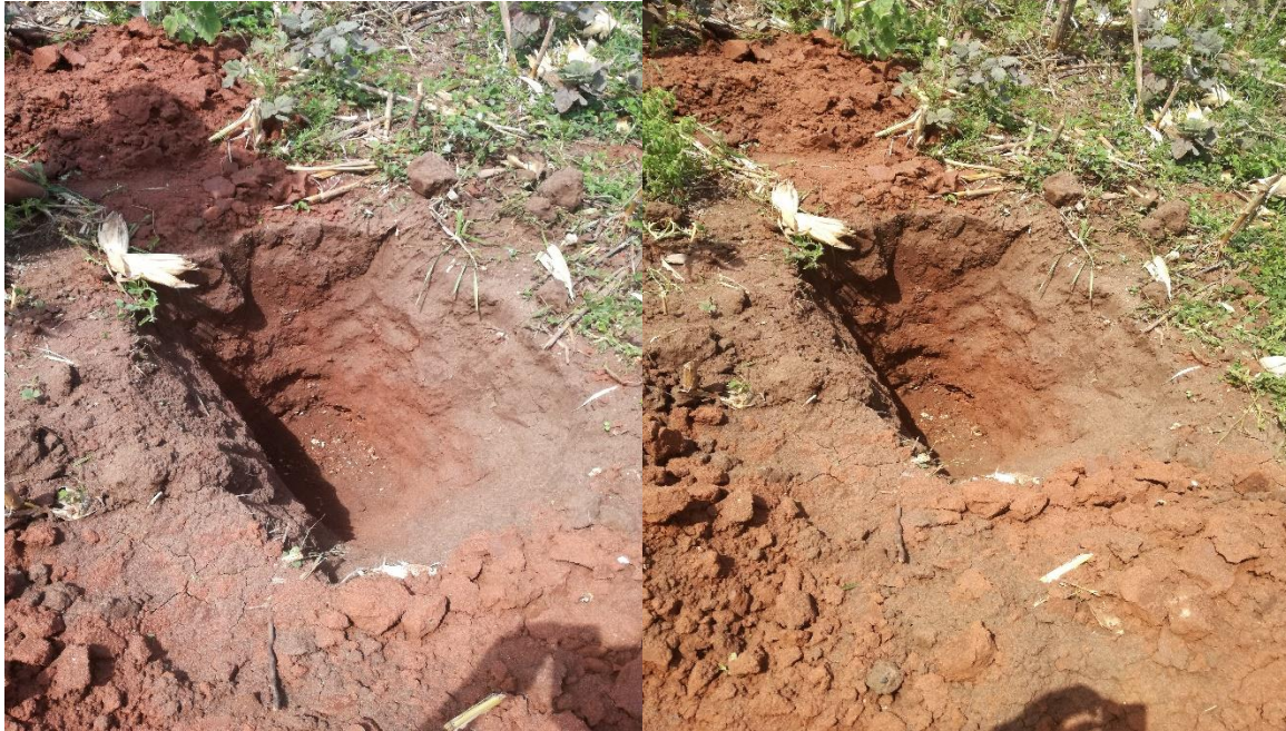
Plate 10.1: Trial pits excavated to determine suitability of gravel for road construction
