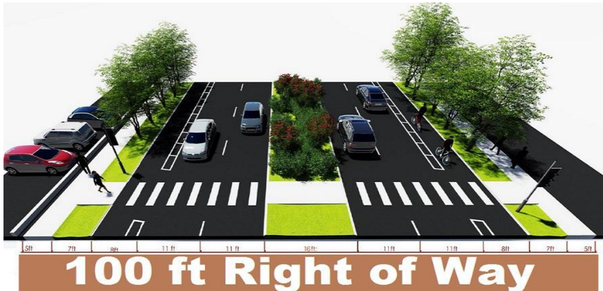
Figure 22: Road Avenue design with environmental incorporations
