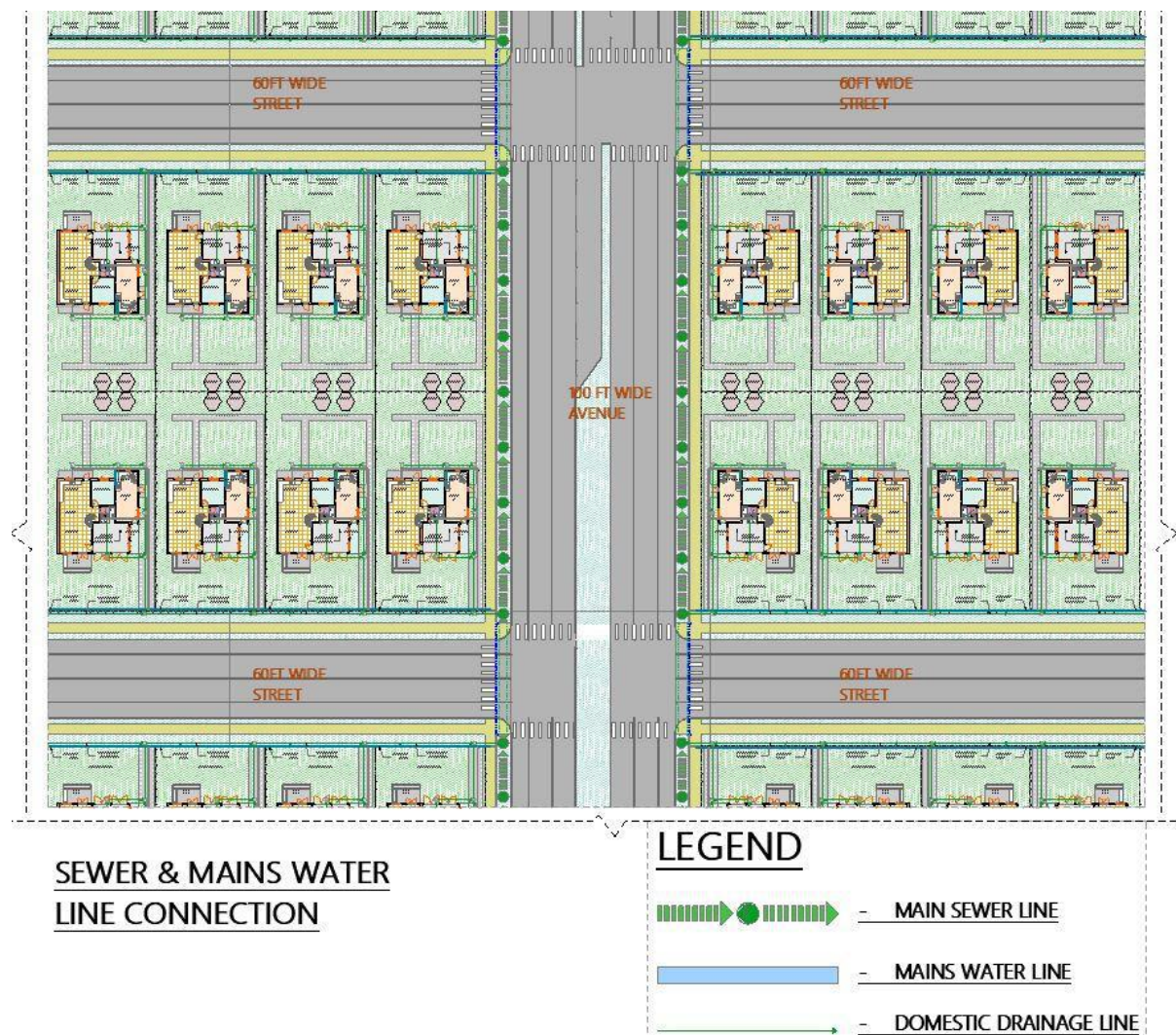
Figure 26: Sewer and Water Lines Infrastructure Design
