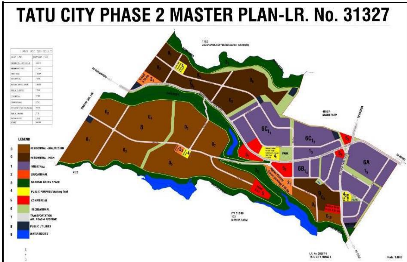
Figure 2.7 Proposed Tatu City Extension (Mchana Estate) Master Plan identifying different land uses : Source (Tatu City, 2019)
