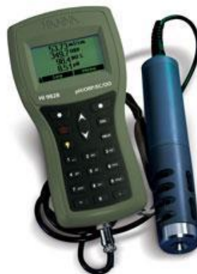
Figure 5: A picture of the Hanna HI 9828 multi-parameter water analyser
