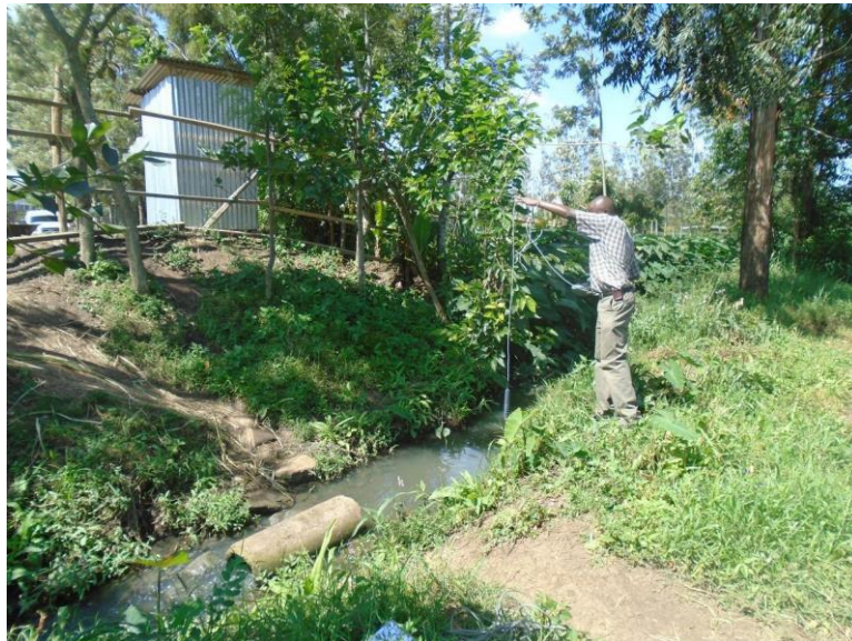
Figure 4: Water quality testing using the Hanna HI 9828
