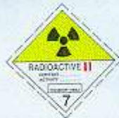
(No. 7B) Category II - Yellow Symbol (trefoil) : black ; Background : upper half yellow with white border, lower half white ; Text (mandatory) : black in lower half of label : 'RADIOACTIVE' 'Contents.....' 'Activity.....' In a black outlined box - 'Transport Index' Two red vertical bars should follow the word 'Radioactive'; Figure '7' in bottom corner
