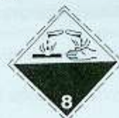
(No. 8) Symbol (liquids, spilling from two glass vessels and attacking a hand and a metal) : black ; Background : upper half white, lower half black with white border ; Figure '8' in white in bottom corner
