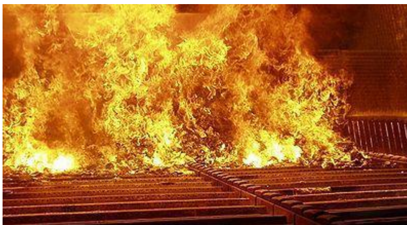
Figure 1. 1Moving Grate Incinerator in operation
