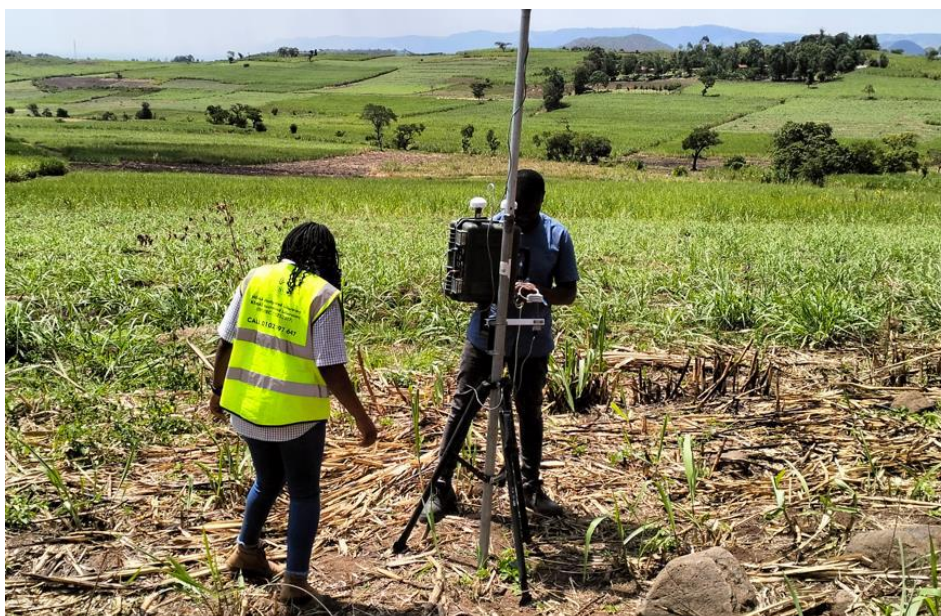
Figure 3.4.3: Ongoing determination of the ambient air quality levels at the proposed Tinderet sugar factory site using HAZ-SCANNER instrument
