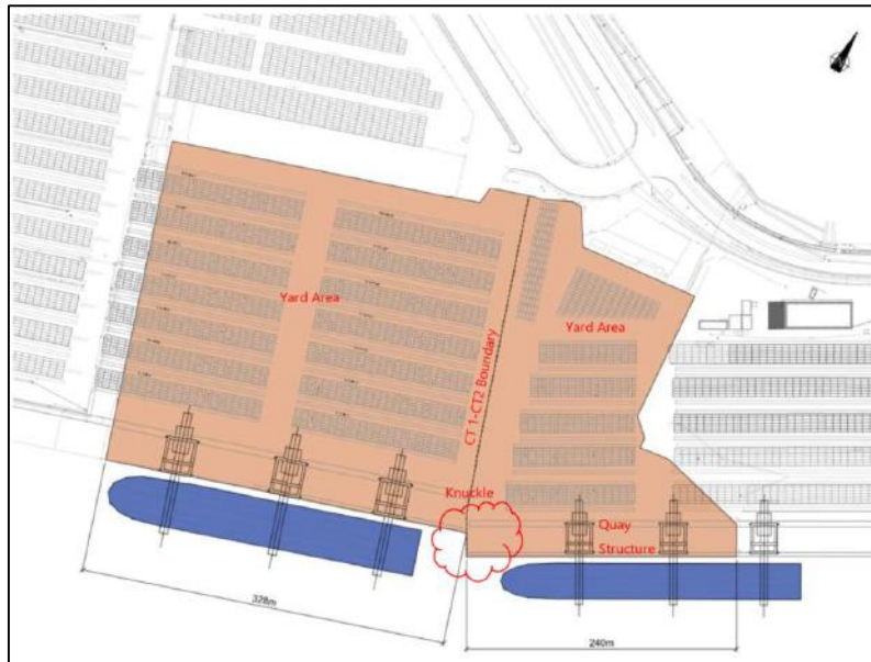
Figure 39 240m quay extension to CT1, 330m extension to CT2, 14.4ha additional yard area
