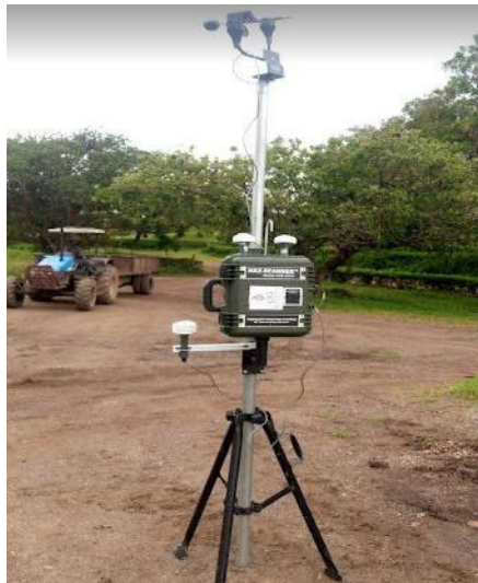
Figure 3.7.3: Ongoing determination of the ambient air quality levels at the proposed Muwariziki Sugar factory site using HAZ-SCANNER instrument
