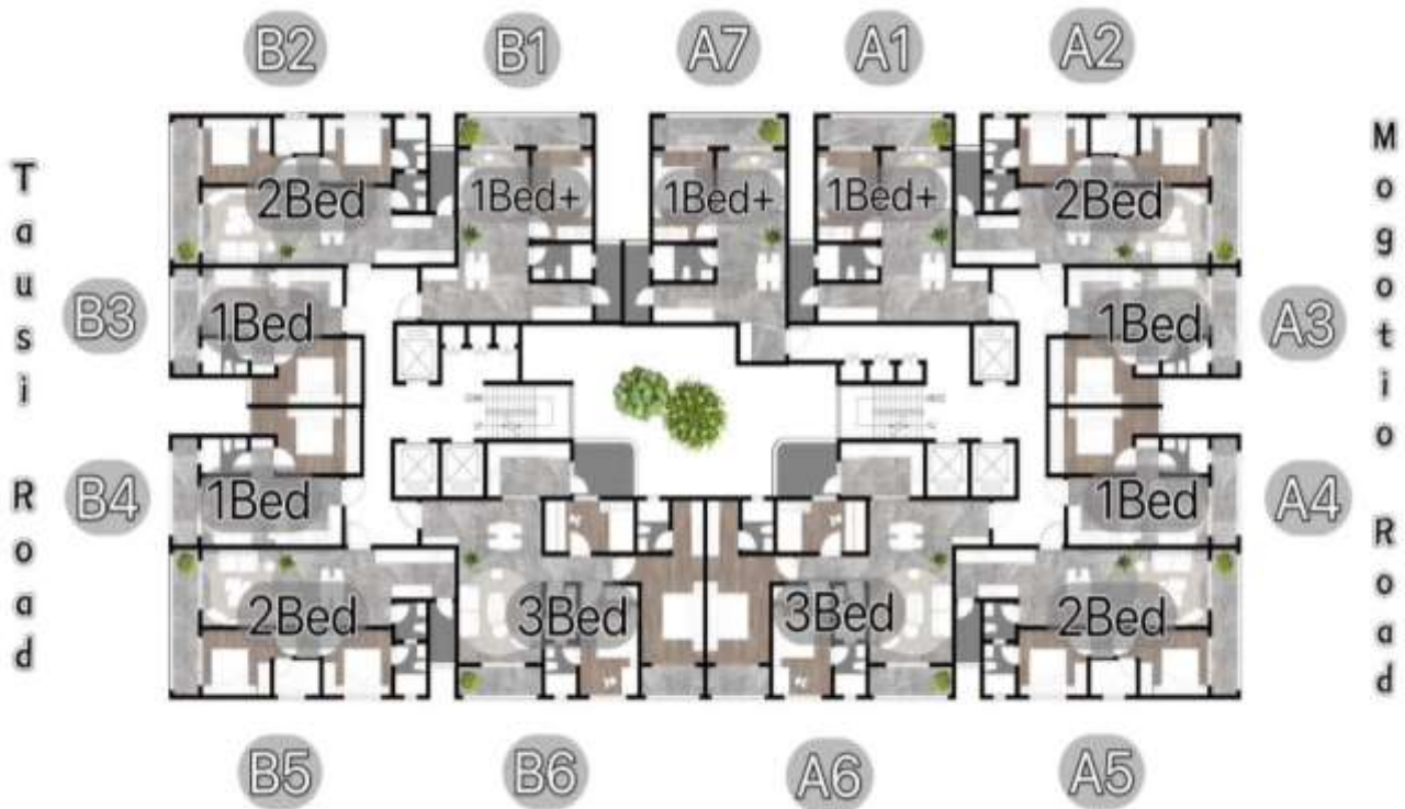
Figure 2: Building floor Layout for the 24 floors
