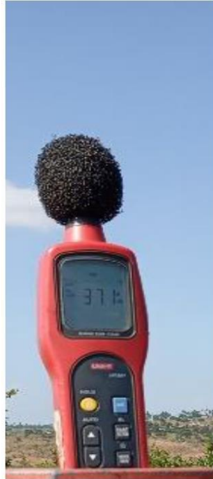
Ongoing diurnal acoustic level measurements at the proposed boundaries (source: Fieldwork May, 2024)
