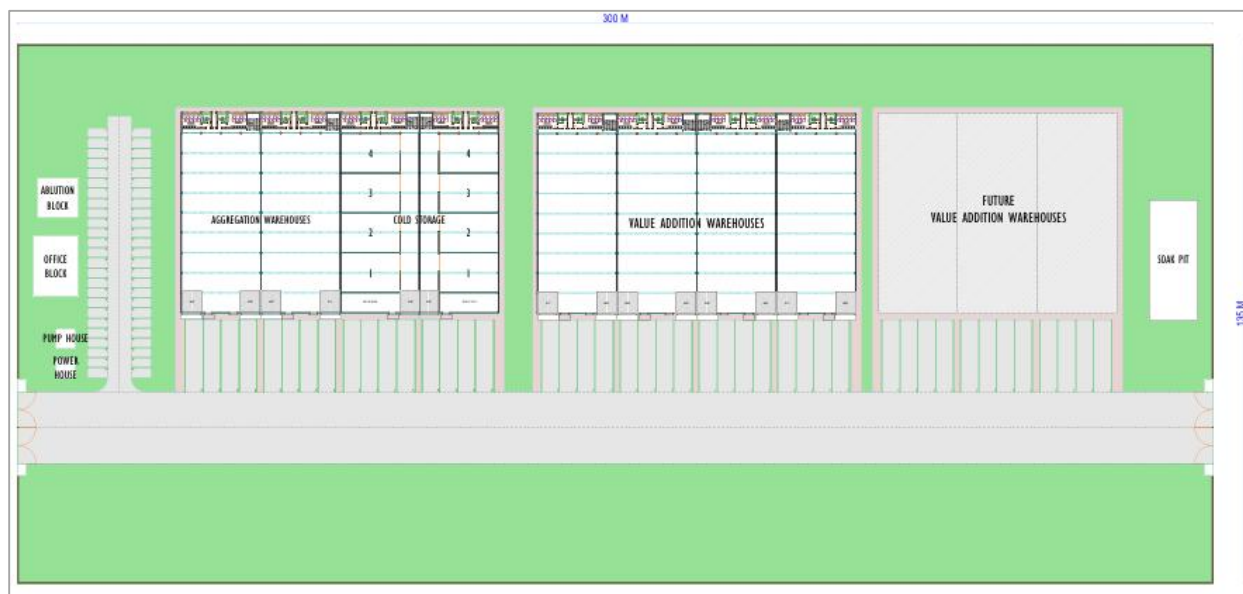
Figure 3: Site layout plan of the proposed CAIPs (Source: Arch. L.M. Mochama)
