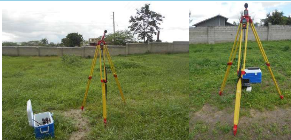
Ongoing diurnal acoustic measurement at the site boundaries
