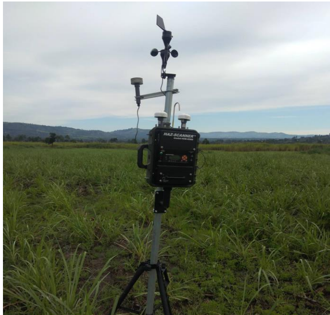
Figure 3.5.2: Ongoing determination of the ambient air quality levels at the proposed Soit sugar factory site using HAZ-SCANNER instrument
