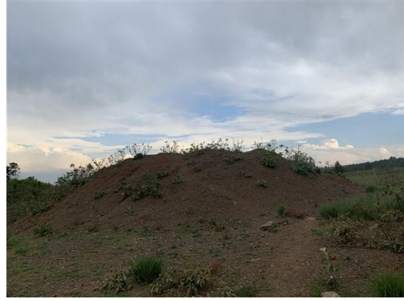
Plate 5-2: Excess overburden stockpiled on site thus exposure to erosion
