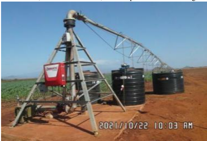
Figure 2-8: Zimmatic 9500P Pivot irrigation system at coordinates 37M 0360888 m E 9615848 m N.
