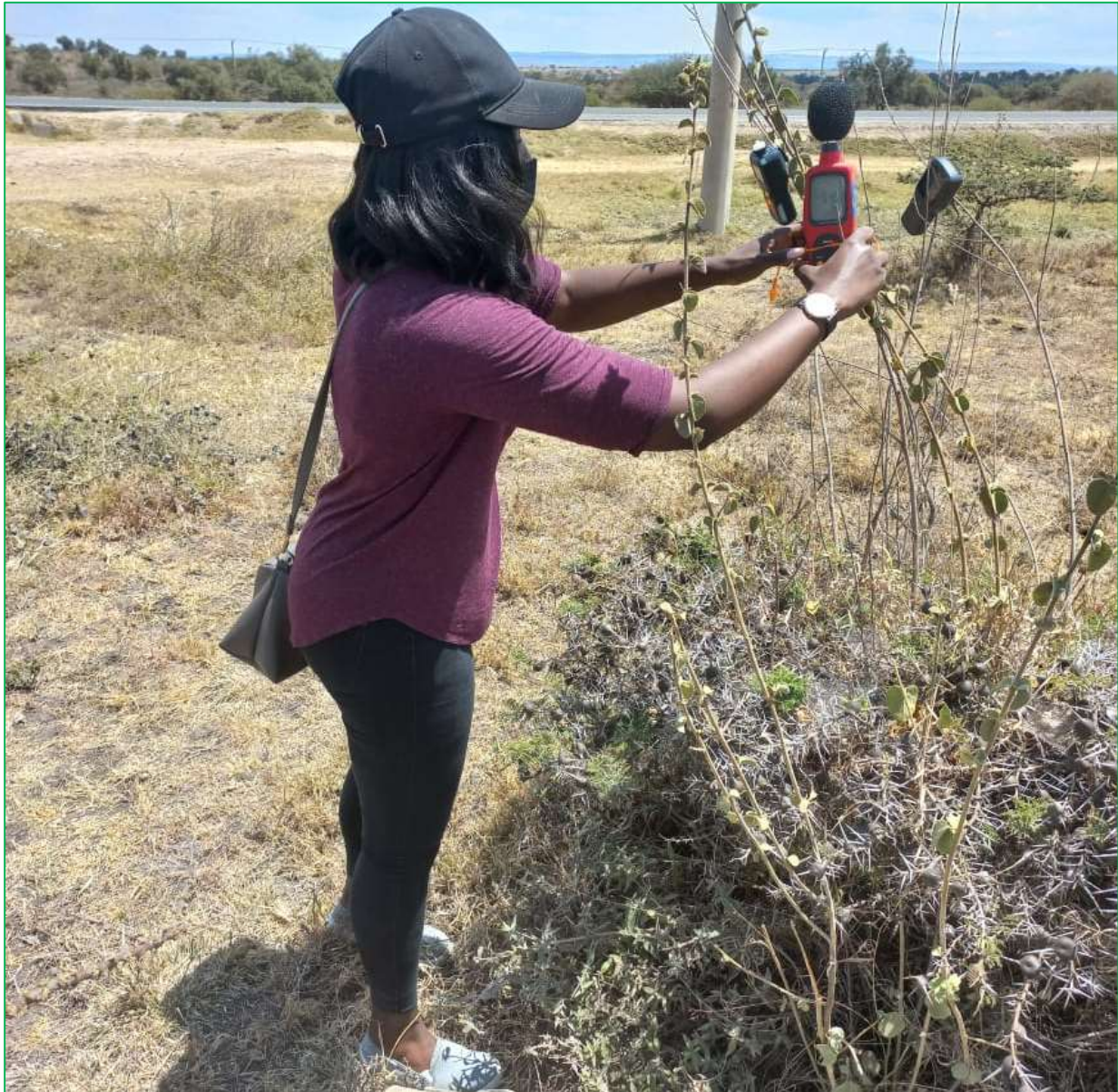
Figure 9: Ambient air quality and noise level monitoring at the proposed project site (Source: Lahvens (K) Limited, August 2021).
