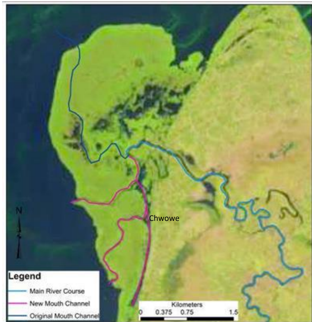
Figure 3: Sondu Miriu River mouth changes in channels from northern to the southern flowing direction as observed through from 1973 to 2021 on satellite images
