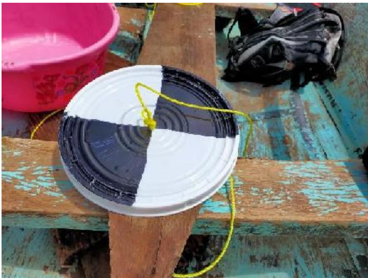
Plate 2: Secchi Disc used for measuring water transparency in the near distance of Sondu Miriu River mouth
