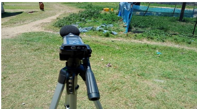
Figure 2: Ongoing noise measurement at Portreiz
