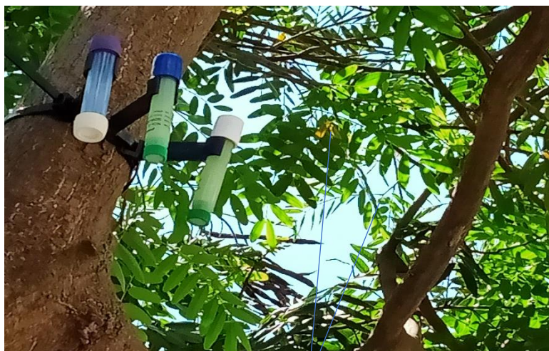
Figure 3: Nitrogen Dioxide measurement in progress
