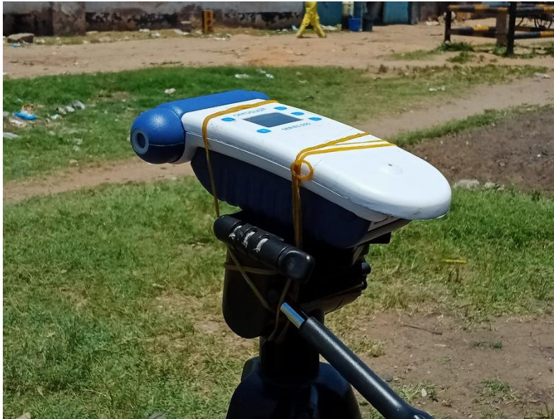
Figure 5: Total Volatile Organic Compounds measurement in progress
