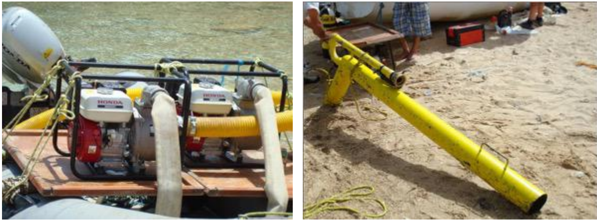
Photo 2-10 Post-cable Laying Equipment
