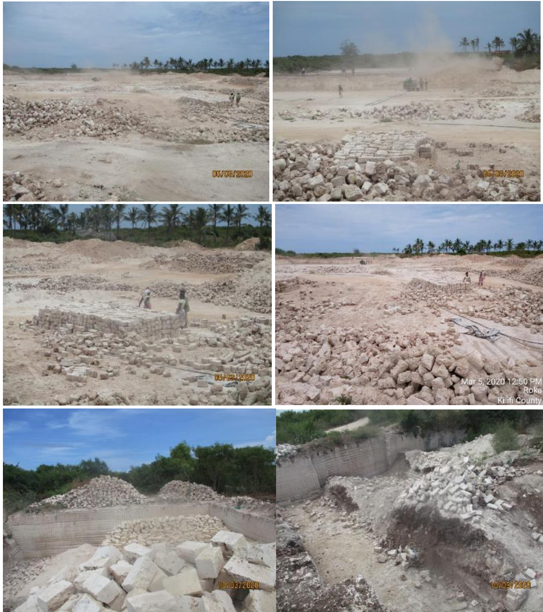
Plate 1: Active machine cut coral limestone quarries adjacent to proposed project site areas
