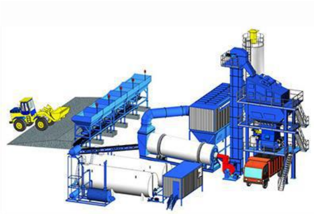
Figure 2: Typical component of an asphalt plant
