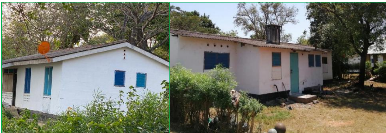
Figure 9: Fisheries staff houses covered with asbestos roofing sheets (Source: Site visit, September 2020).
