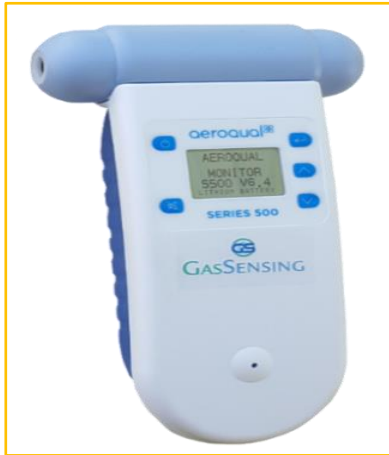
Figure 5: A portable Seroquel series 500 used in obtaining baseline air quality measurements at the proposed project site.
