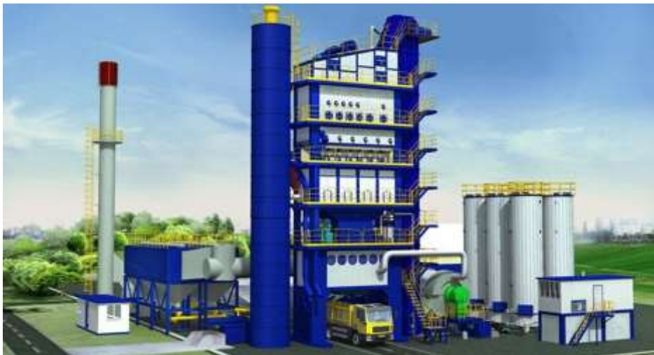
Figure 10: Impression of Asphalt plant
