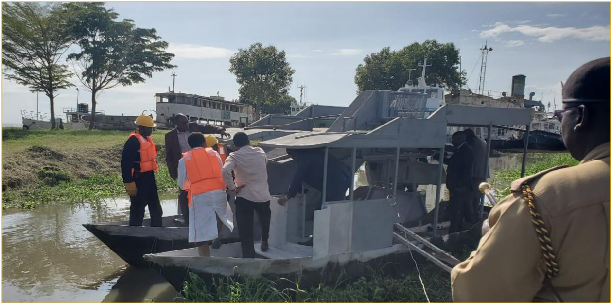
Figure 52. A water hyacinth harvester built by Kisumu Polytechnic at the Port in November 2019 (Source: KPA, 2019)
