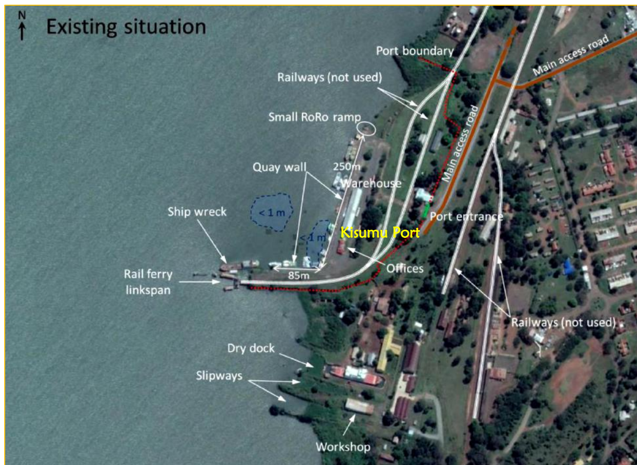
Figure 3. The existing facilities at Kisumu Port (Source: Kenya Ports Authority Master plan, 2019).
