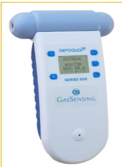
Figure 16. A portable (Aeroqual 500 - Series) used in obtaining baseline air quality measurements at Kisumu Port.
