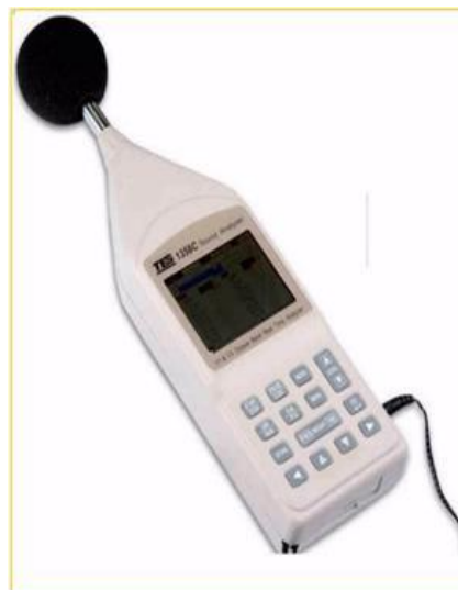
Figure 17. Noise level meter (Model TES 1358 C) used in obtaining baseline noise levels at Kisumu Port.
