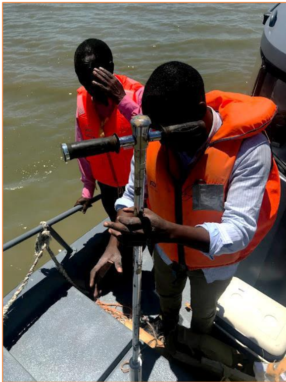
Figure 15. The Auger Sampler used in collection of sediments at River Kisat Estuary and the Kisumu Port Pier area (Source: Site visit, November 2019).
