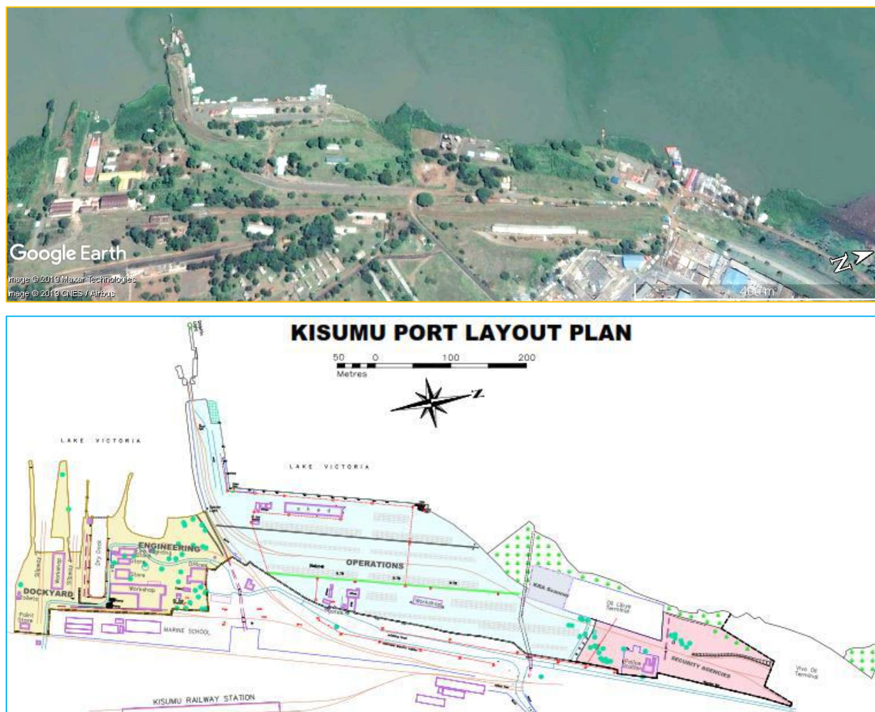
Figure 4. Top, the status of Kisumu Port in December 2017 and; bottom the layout of the proposed Kisumu Port revitalization works and components (Source: Kenya Ports Authority, 2019).
