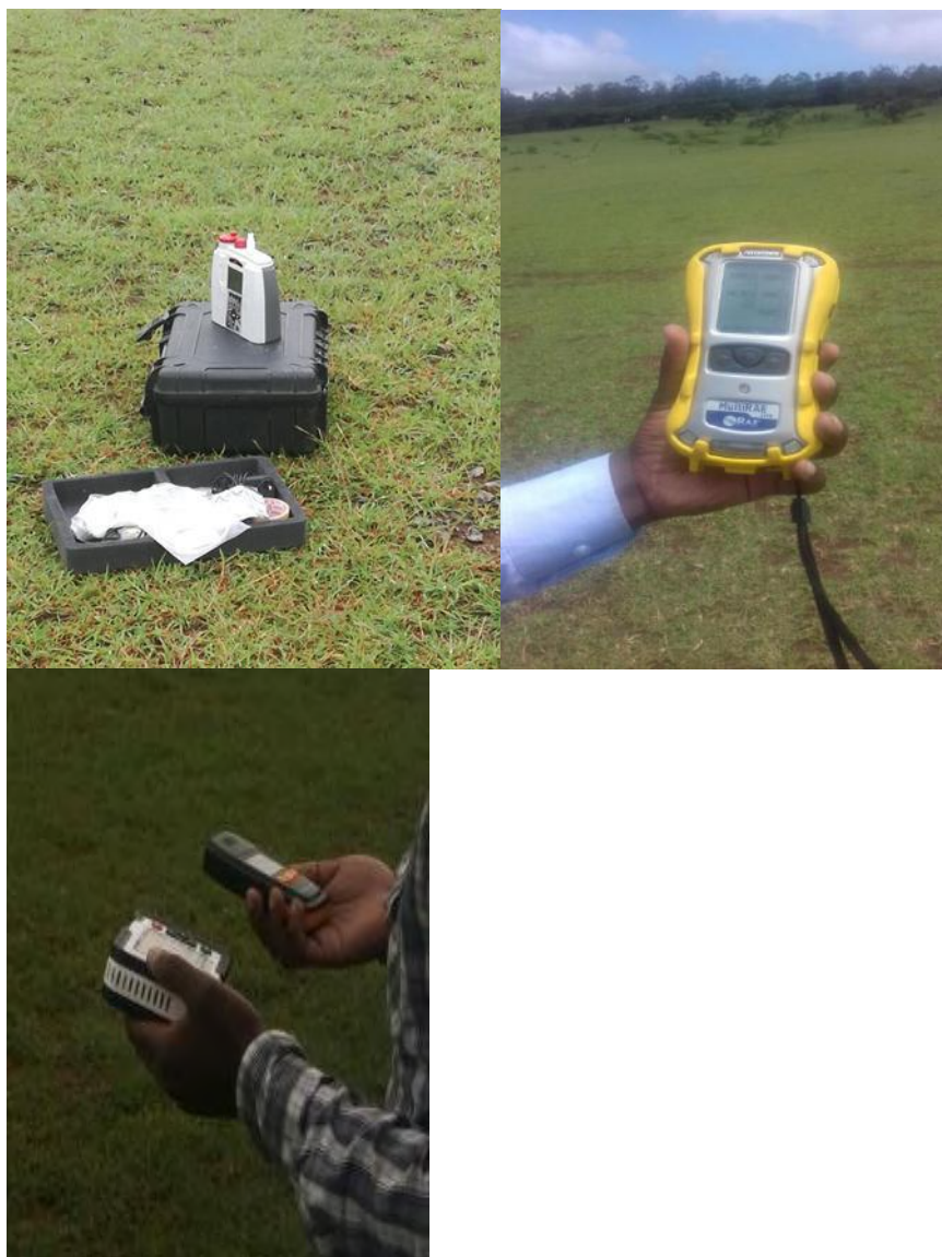
Fig of meters used, MultiRae, CO meter, EVM analyzer, manufactured by the 3M Company
