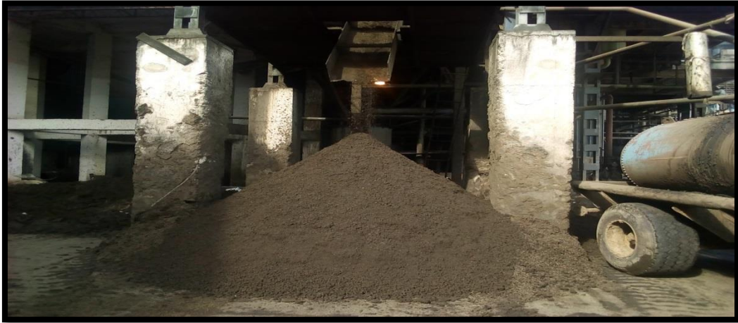
Plate 12: Filter Mud from the factory that shall be used as one of the raw materials for the new bio fertilizer factory.
