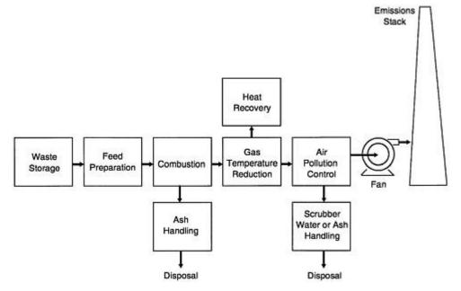
Figure 4: proposed waste-incineration facility schematic
