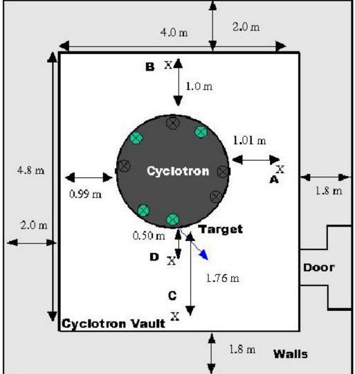
The walls to the Cyclotron are two meters thick. They will be constructed as per the required professional guidelines. Further the Cyclotron will be at least one meter from the walls. Radiation effects will therefore be minimised
