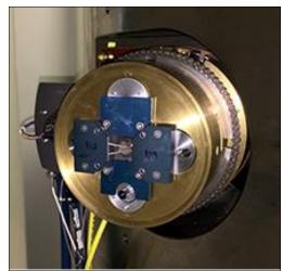
The spiral beam of particles widens and hits one of the two targets located on either side of the vacuum chamber. The cyclotron at HSC Winnipeg contains eight such targets in two carousels. Cyclotron beams are used to bombard other atoms to produce short-lived positron-emitting medical isotopes suitable for use with the PET scanner.
