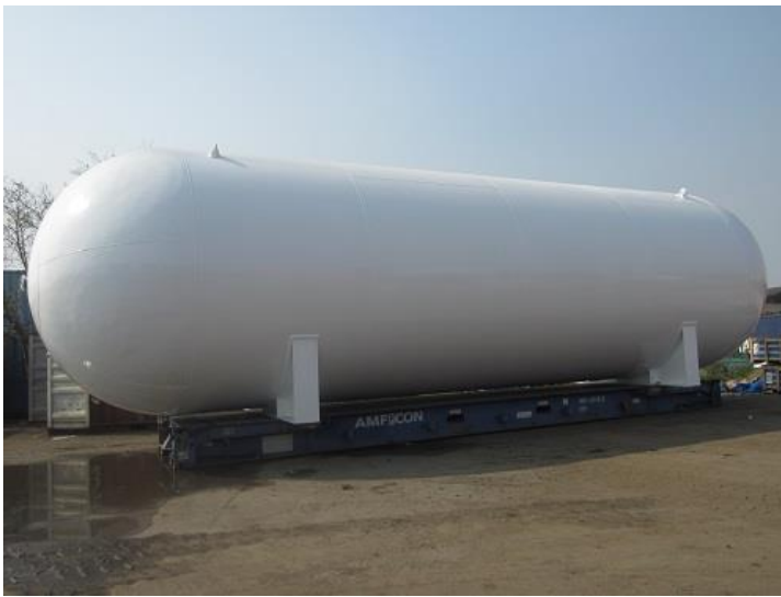
Figure 8: An image of LPG Cylindrical Tank
