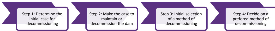
Figure 8-2 Steps in dam decommissioning
