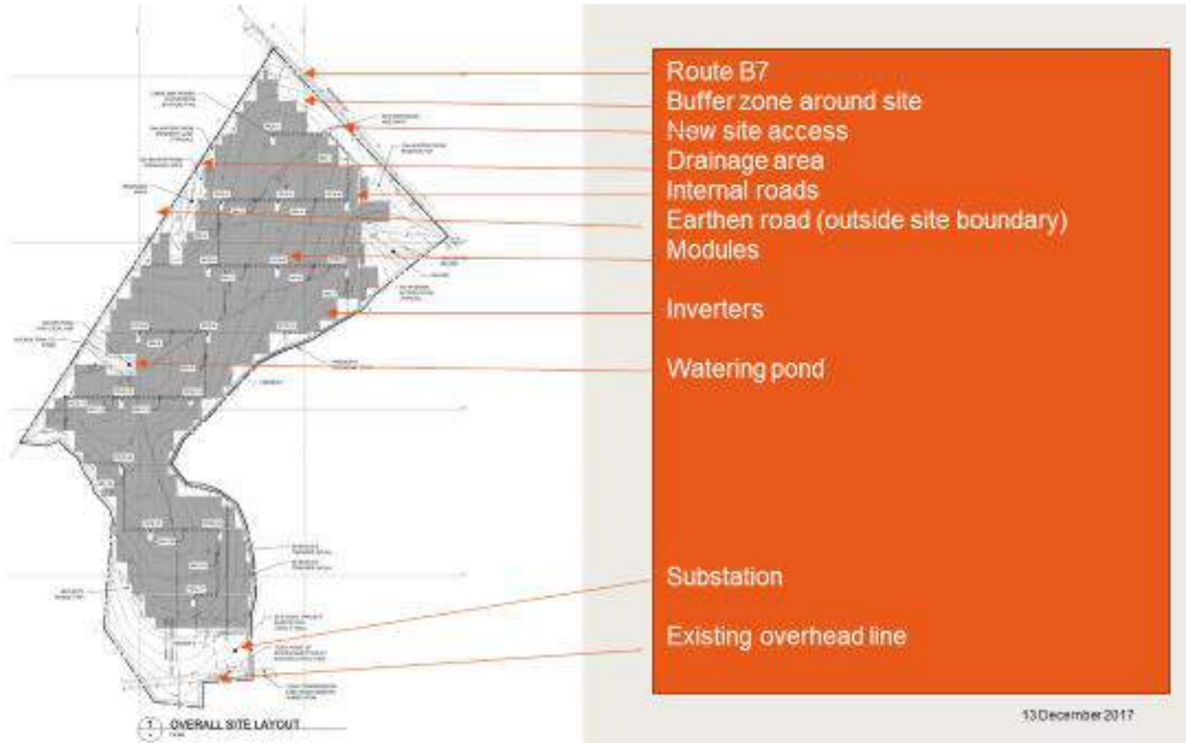
Figure 4: Preliminary representative plant layout
