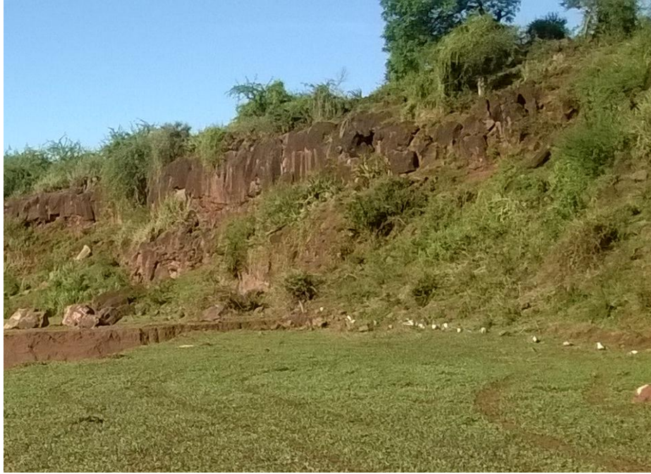
Figure 3:- Basalt cliff on the right bank of Lewa river around the dam axis. The rock exhibits moderate jointing.
