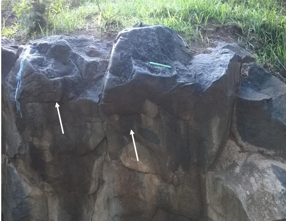
Figure 6:- Jointed basalt rock on the left bank. White arrows show the joint
