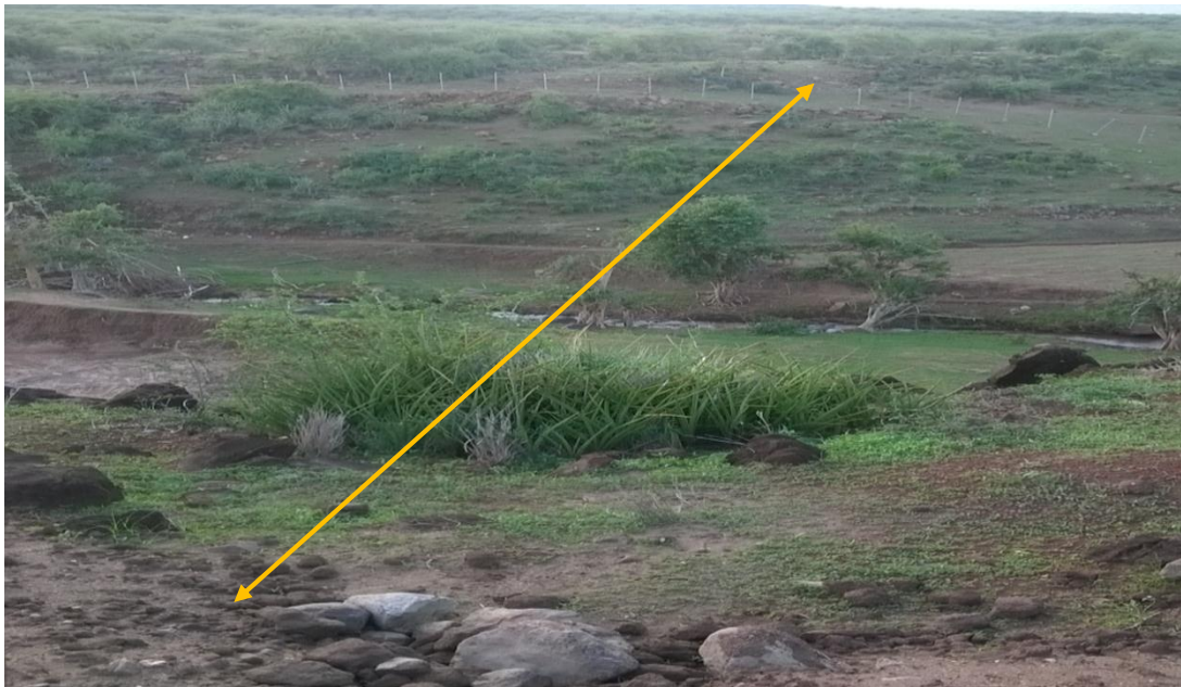
Fig 3.: Stony soils on basalt on the right bank in the foreground of the picture. The left bank in the background shows a thick layer of bouldery volcanic material probably overlying jointed basaltic rock. The approximate orientation of dam axis is shown by yellow double arrow.
