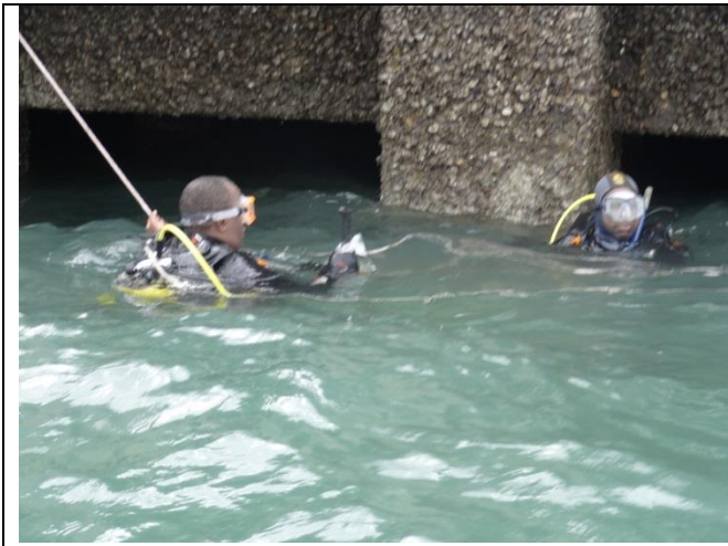
Plate 5.3A: use of ropes to access sea-floor beneath wharfs due to poor visibility – purpose: for sub-marine-sampling
