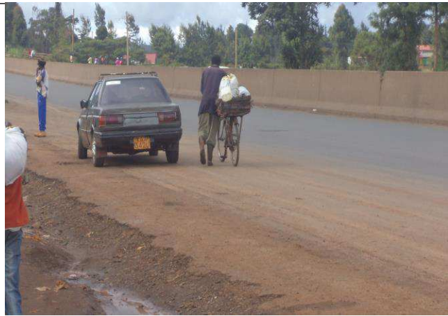
Conflict between Motorized traffic (MT) and Non Motorized Traffic (NMT) due to lack of NMT facilities such as cycle tracks and pedestrian walkways
