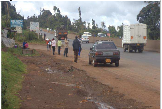
Conflict between Motorized traffic (MT) and Non Motorized Traffic (NMT) due to lack of NMT facilities such as cycle tracks and pedestrian walkways
